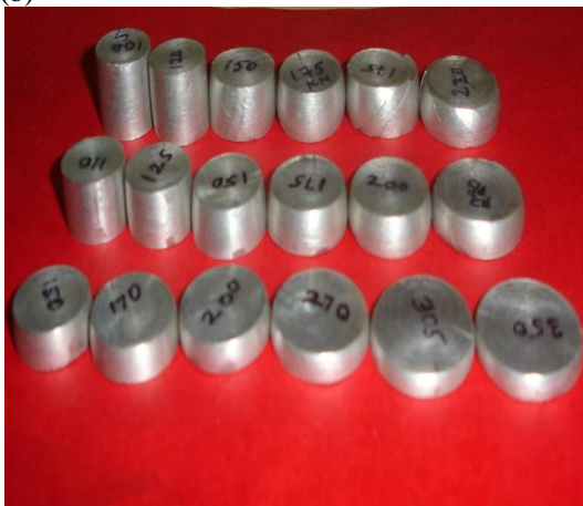
Fig 1: Cylindrical specimens of different aspect ratios (a) before deformation (b) after deformation
